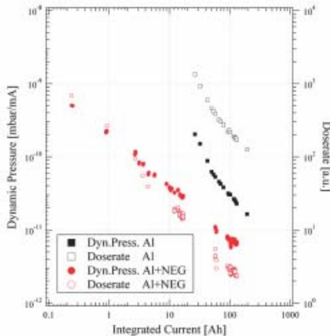
*Comparison between the dynamic pressure and the bremsstrahlung of two aluminum vacuum chambers for Insertion Device, one with an IntegraTorr SNEG coating and the other one without, installed at ELETTRA*
