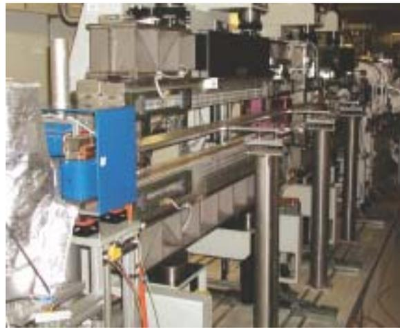
*Aluminum Insertion Device vacuum chamber with IntegraTorr SNEG coating.*
