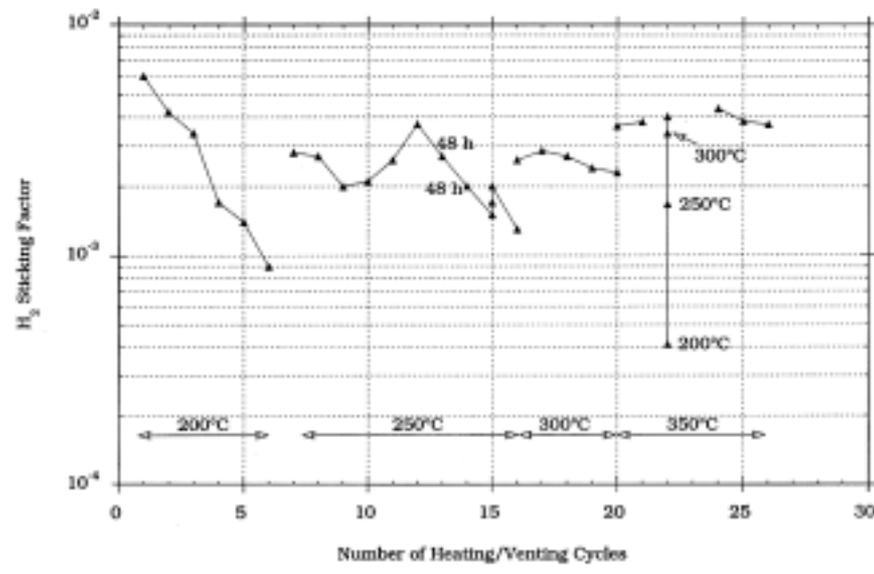
Variation of the H<sub>2</sub> sticking factor for a 5 m thick Ti Zr V film as a function of the number of activation-air-venting cycles.
