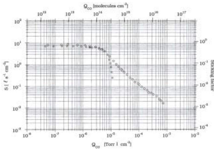
Variation of pumping speed for CO as a function of the pumped quantity for a Ti Zr V film (squares) and for a very rough coating (circles). CERN data.
