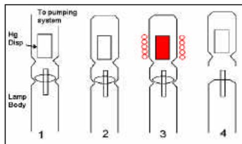
Fig.1 – Double tip-off technology for CCFL production
