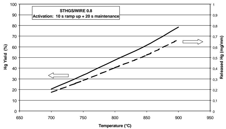
Fig. 3: Typical Hg Yield curve for a Sthgs/Wire
