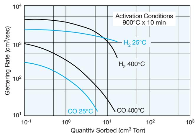
Figure 7: Sorption curves of St 171/LHI/4-7/200 for CO and H<sub>2</sub> at room temperature and at 400°C after an activation at 900°C for 10 minutes.
