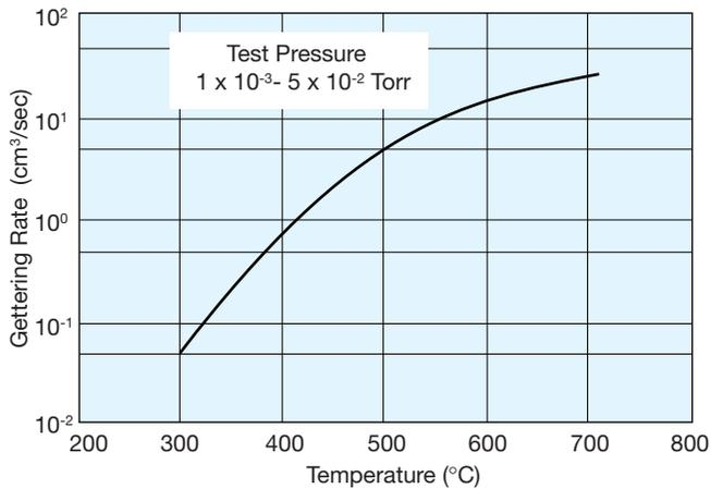
Figure 8: The gettering rates of St 171/LHI/4-7/200 for CH<sub>4</sub> at different temperatures.
