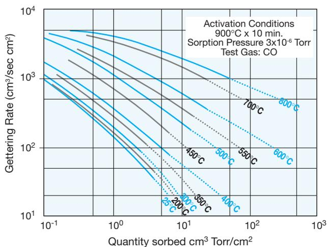
Figure 5: A family of sorption curves for CO at different operating temperatures after an activation at 900°C for 10 minutes.
