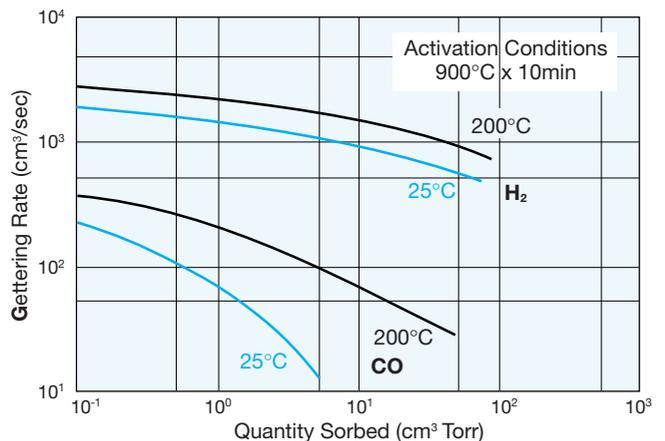
Figure 14: St 172/LHI/4-7/200 sorption curves for CO and H<sub>2</sub> at room temperature and 200°C after an activation at 900°C for 10 minutes.
