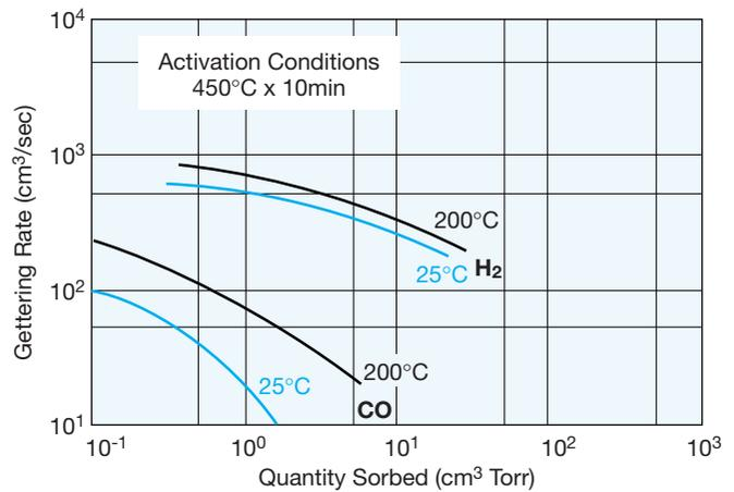
Figure 13: St 172/LHI/4-7/200 sorption curves for CO and H<sub>2</sub> at room temperature and 200°C after an activation at 450°C.
