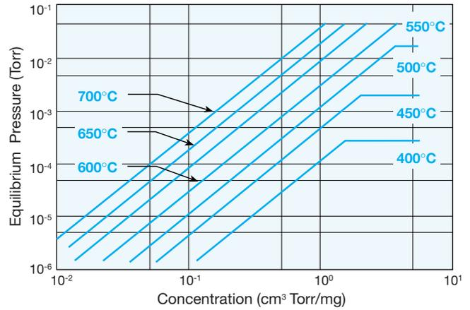
Figure 12: The H<sub>2</sub> equilibrium pressures of St 172 as a function of the H<sub>2</sub> concentration in the gettering material at different working temperatures.
