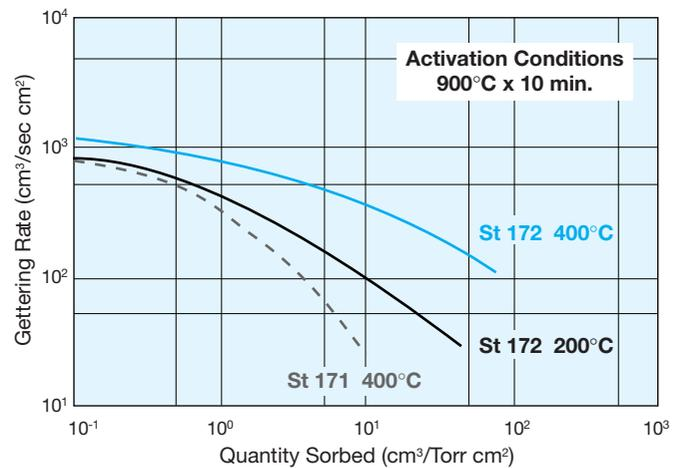
Figure 19: Comparison of St 171 and St 172 for CO at different sorption temperatures with activation conditions of 900°C for 10 minutes.
