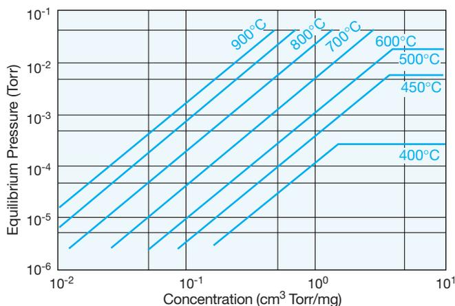
Figure 6: The H<sub>2</sub> equilibrium pressures of St 171 as a function of the H<sub>2</sub> concentration in the gettering material at different working temperatures.
