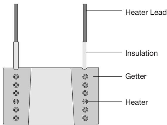
Figure 2: A typical configuration of a zirconium based sintered porous getter.
