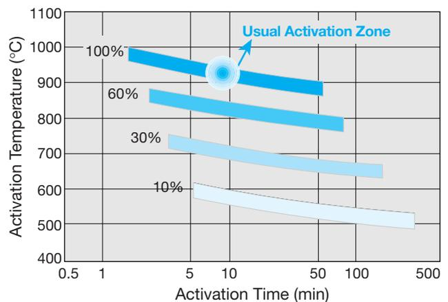
Figure 4: The gettinger efficiency of St171 (expressed as a percentage of the initial gettinger rate of a fully activated getter) after various activation conditions.
