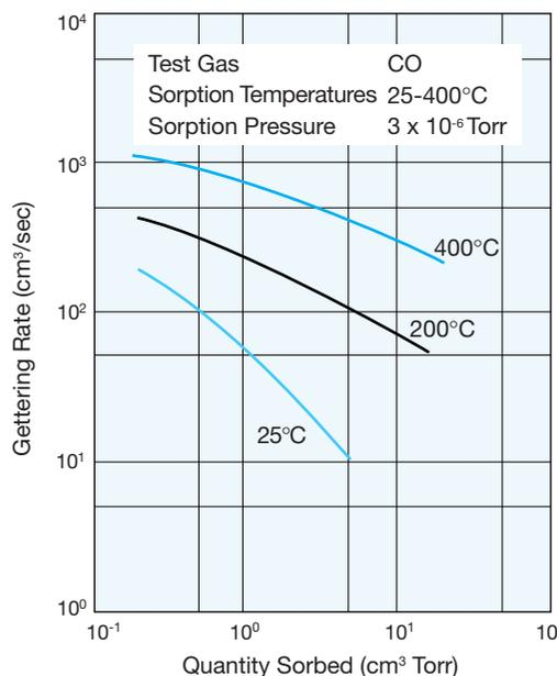
Figure 11: St 172/LHI/4-7/200 sorption curves for CO at room temperature, 200°C and 400°C after an activation at 900°C for 10 minutes.
