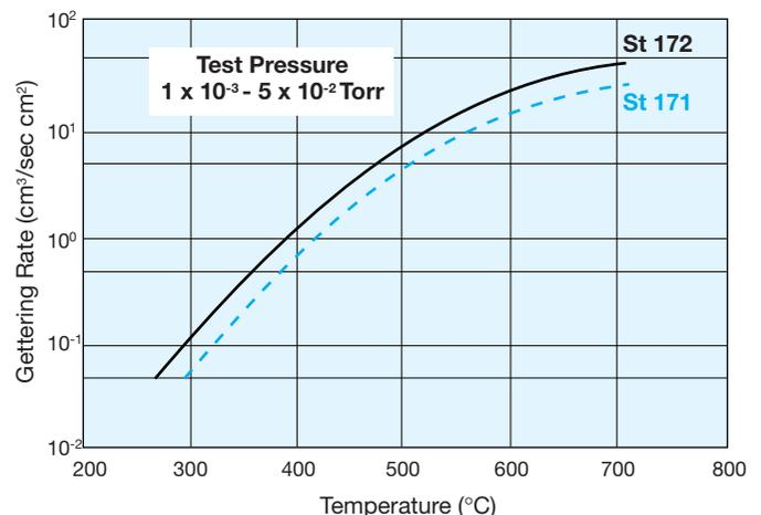
Figure 20: Comparison of St 171 and St 172 for CH<sub>4</sub> with a test pressure of 1 x 10<sup>-3</sup> - 5 x 10<sup>-2</sup> Torr.
