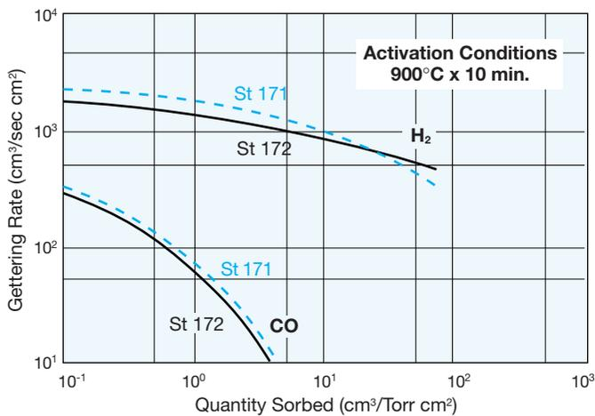
Figure 17: Room temperature comparison of St 171 and St 172 with activation conditions of 900°C for 10 minutes.
