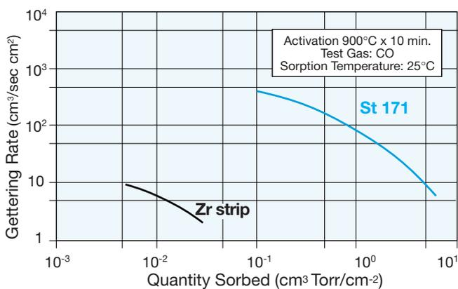
Figure 1: A comparison of sorption characteristics for a Zr strip and a St 171 sintered porous Zr-based getter.
