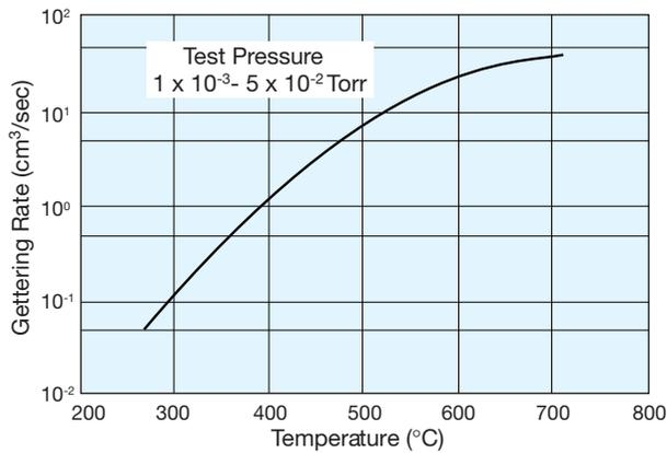
Figure 15: The St 172/LHI/4-7/200 gettering rates for CH<sub>4</sub> at different temperatures.
