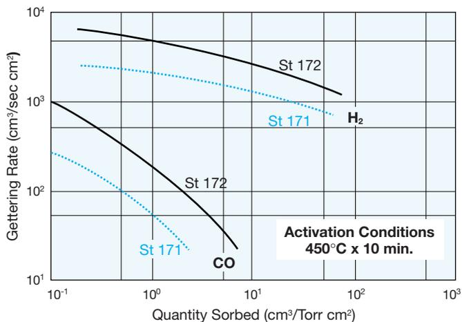
Figure 18: Room temperature comparison of St 171 and St 172 with activation conditions of 450°C for 10 minutes.
