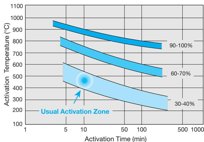
Figure 10: The gettering efficiency of St 172 (expressed as a percentage of the initial gettering rate of a fully activated getter) after various heating treatments.
