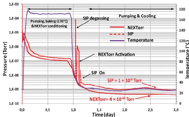
Figure 4: Comparison of the pump-down experiments with combination and conventional SIP pumps (baking 170°C for 24 hours).
