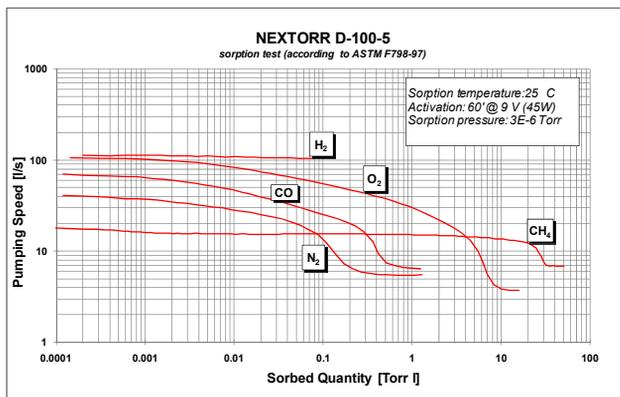
Figure 2: Typical sorption curves of the NEX Torr<sup>®</sup> D100-5.
