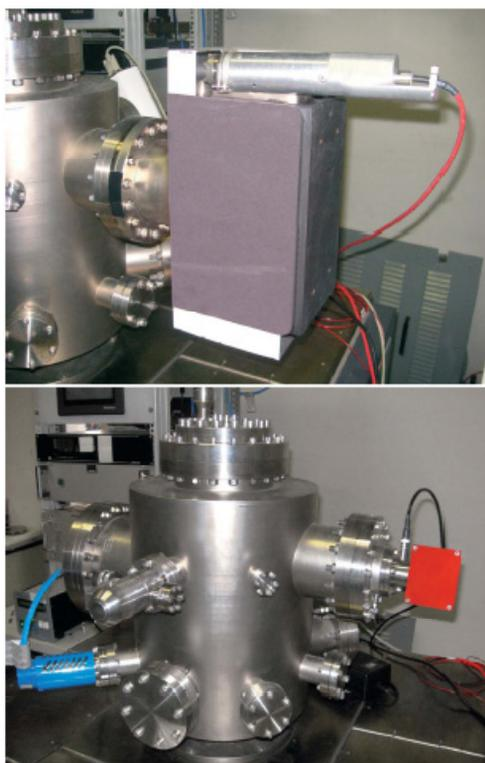
Figure 3: Picture of the UHV test bench with the SIP and the NEX Torr<sup>®</sup> D100-5 installed.
