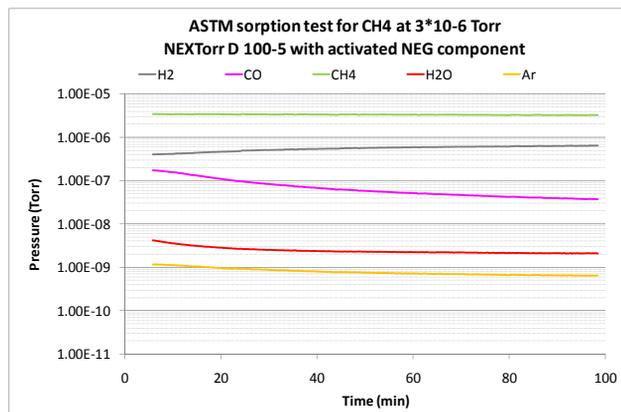
Figure 7: Gas composition during the sorption of methane with active NEG.
