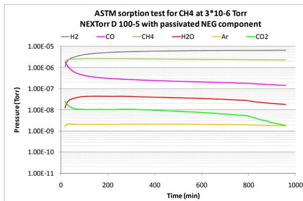
Figure 6: Gas composition during the sorption of methane with passivated NEG element.
