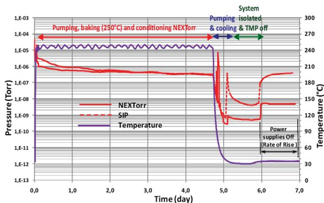
Figure 5: Comparison of the pump-down experiments with combination and conventional SIP (baking 250 °C for 110 hours).
